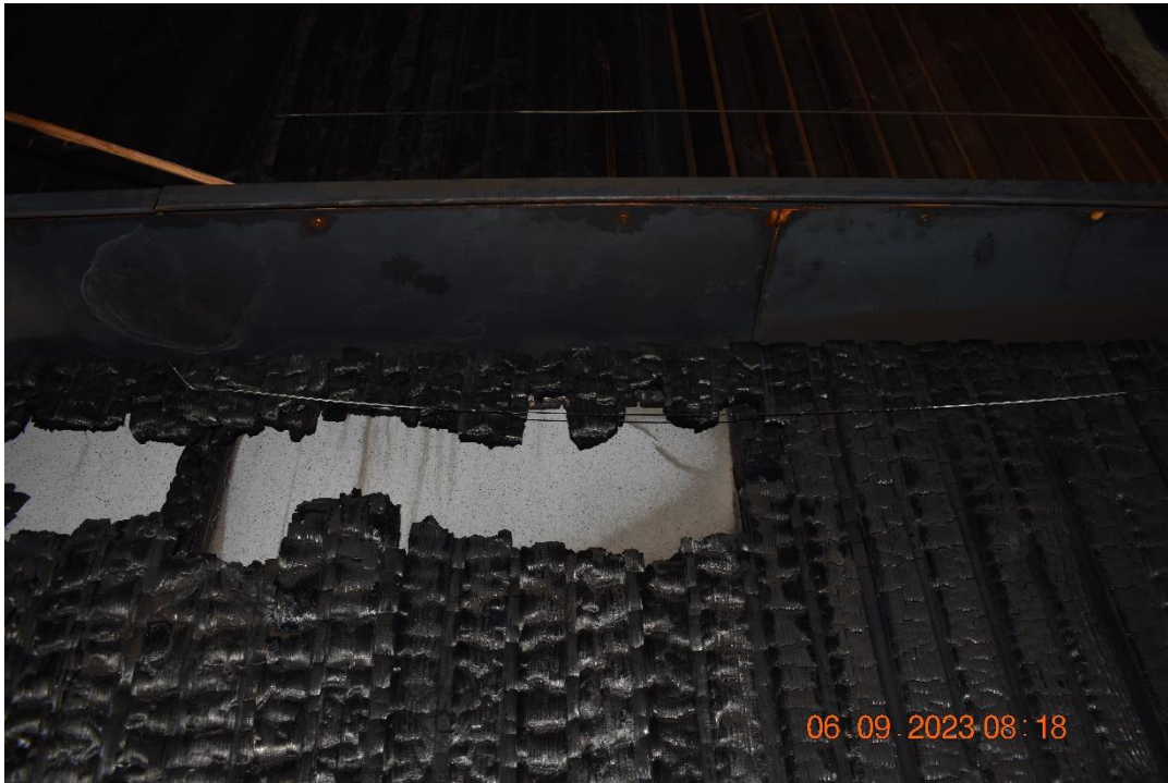
Photo No. 25 Test specimen after the test. Detail photo of cladding above the fire chamber.
