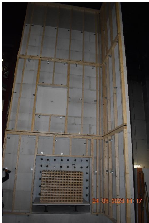
Photo No. 2 Prefabricated cassettes mounted on the façade rig.
