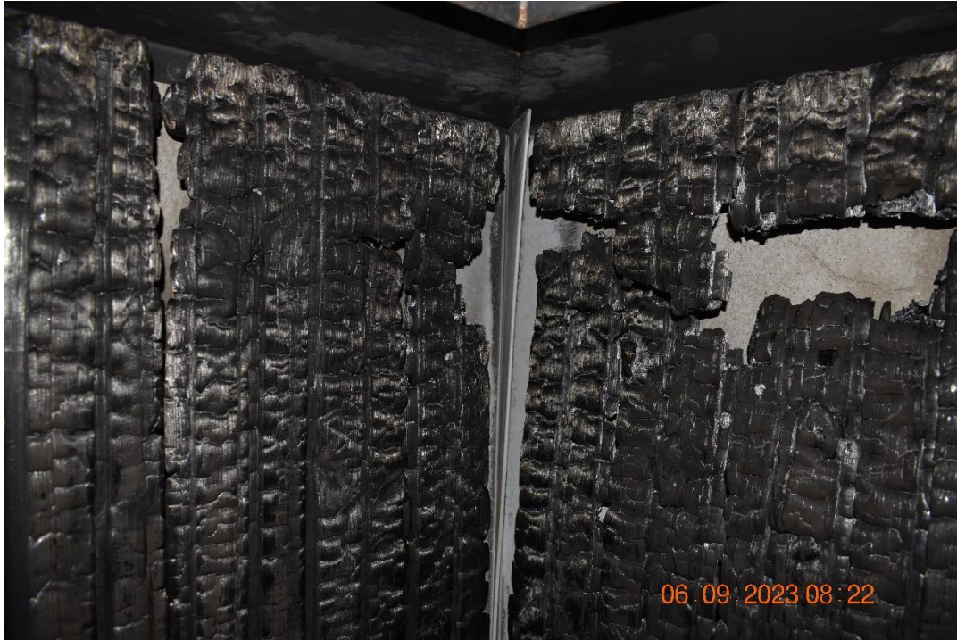
Photo No. 23 Test specimen after the test. Detail photo of cladding in the corner below the first flame breaker.
