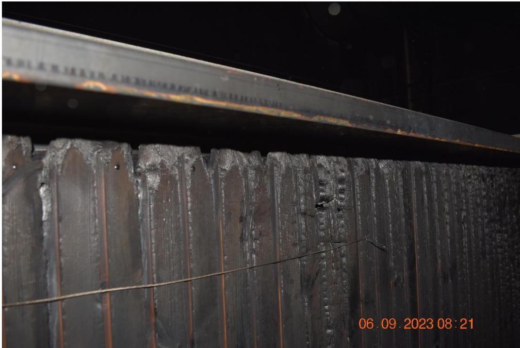
Photo No. 27 Test specimen after the test. Top of main façade.
